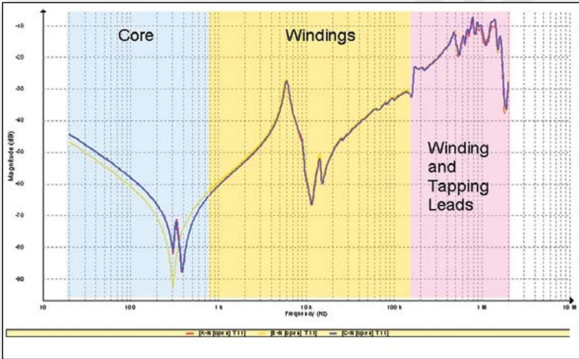
This graph shows a typical trace for a Star-Delta transformer with the LV open circuited. The highlighted regions indicate the parts of the transformer predominantly affecting the different frequency ranges
