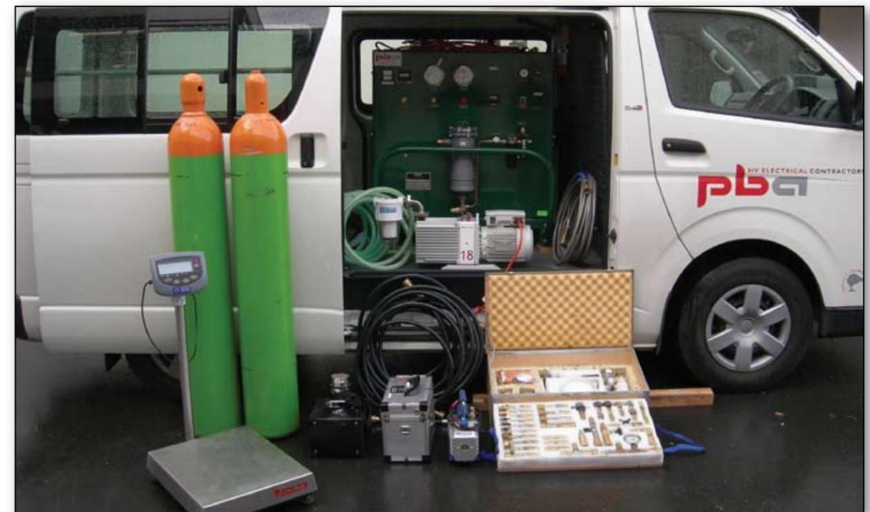
PBA's Enervac GRU-6 SF<sub>6</sub> Gas Cart and SF<sub>6</sub> accessories are easily transported in our vans.
